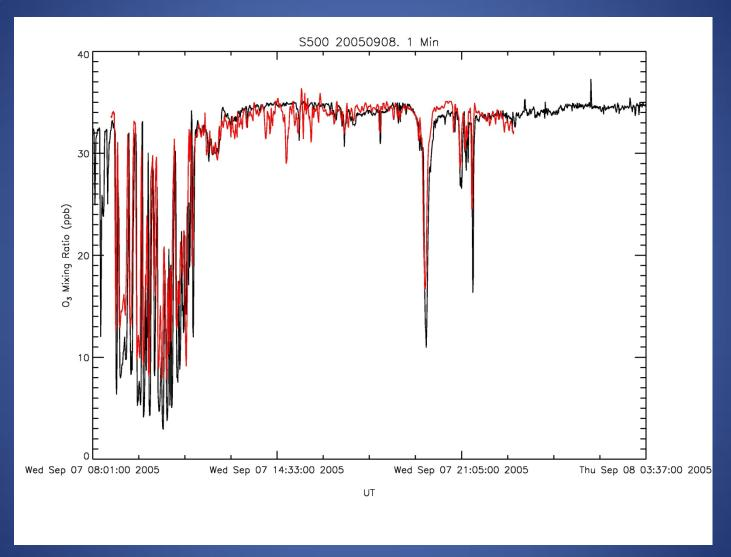
Comparison of measurements from the ozone sensor (red curve) with the Thermo Environmental 49C ozone instrument at McMurdo Station, Antarctica (black curve)
